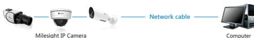
Figure 2-1-1 Connect the camera to the PC directly
