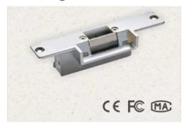
The electric strike lock features an embedded installation with the electromagnetic part being concealed in the door. Made of high quality magnetic materials and using special technology processes, it won't retain residual magnetism ensuring optimal long-term functionality. It supports 90-degree door openings. Our electric strike uses hardened stainless steel and can bear 500kg impact pressure.
