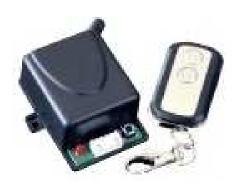
Our remote control is designed for access control applications with the 600lbs MDSM Electromagnetic Lock. The signal can easily penetrate walls and uses Rolling code chip technology.
